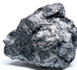
Ore from Sri Lanka: This ore features a special structure and a high graphite content of up to 99%
